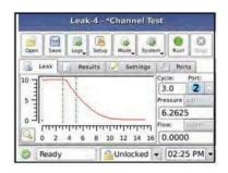
When the leak test is run, you can select a real-time graphic display of the ongoing test that will, upon completion of the test, show the test result (accept/reject/decay).
