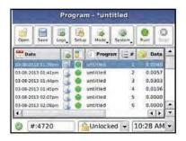
With the Worker Integra leak tester you can create and store testprograms associated with your products.me instrument can be locked so the parameters cannot be accidentally changed.
